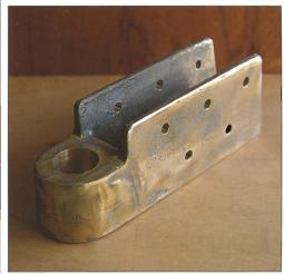
is the hefty bronze gudgeon that foots the rudder. One of the best things you can't see here: the reverse transom opens to release the life raft right into the water. No need to cart around the weighty thing on deck—a brutal task in a presumably brutal situation. First-class offshore thinking.
