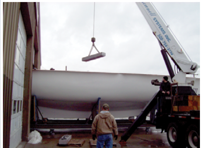
(left) Shannon 53 HPS Hull #1 now located in Charleston, SC (top right) Shoveling the ice and snow from the decks of Shannon 53PHS Hull #3 while on a winter offshore delivery south (bottom right) Lowering the lead ballast into Hull #4
